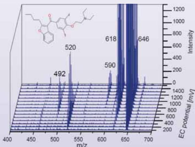
Oxidative "fingerprint" (MS Voltammogram) of Amiodarone (*antiarrhythmic agent*) m/z 646 and its major oxidative metabolites m/z 618, 590, 520 and 492 generated by on-line Electrochemistry-MS using the ROXY EC system equipped with  $\mu$ -PrepCell2.0 and connected to an MS. Total experimental time 15 min.
