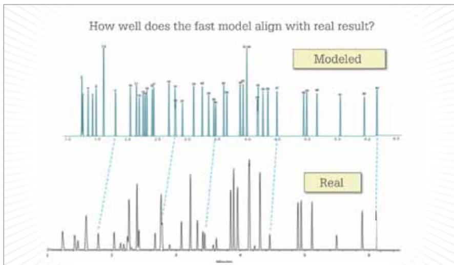
Figure 1. A modeled chromatogram of VOC versus the real result.
