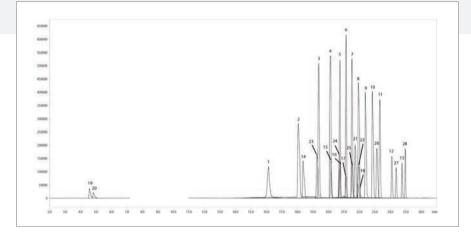
This application note shows the analysis of 28 PFAS in human serum, based on Nakayama et al.'s study (1). An automated solid phase extraction (SPE) system was coupled to an online SPE columnswitching LC-MS/MS method. Anionexchanging scrubber columns were placed downstream of the LC pumps A, C and D in order to eliminate possible contamination from the system. In short, a YMC-Triart C18 column when used as the analytical column shows excellent results for this sensitive analysis.
