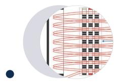
High Resolution Multi-Reflecting Time-of-Flight Mass Analyzer with Folded Flight Path<sup>®</sup>
