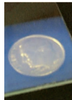
Fig 1. (Top) Field-emission SEM image of ordered film of silica spheres (200 nm) prepared in our lab in 2002. This is a side view of cleaved sample that was 4 \mu\text{m} thick. (Right) Photograph from 2002 of a typical microscope slide coated with silica colloidal crystal from the same particle size. The blue color is from Bragg diffraction, and the dime behind the slide shows that these materials are optically transparent. Reprinted with permission (1).
