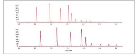
Fig 2: Separation of alkylphenones in constant pressure mode (1000 bar) (upper trace) and constant flow mode (0.6 ml/min) (lower trace, red = constant pressure vs virtual time, blue = constant flow vs real time).
