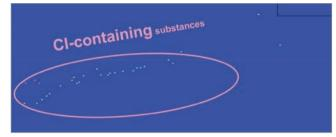
Figure 3. Two dimensional GCxGC-EI-TOF-MS chromatogram. Scripting software detects isotopic features of chlorinated analytes which are filtered from the raw data and depicted as dots. Spectra retrieved from a dots can then be searched against the halogenated compounds from a generic library (e.g. NIST) to aid in the identification.
