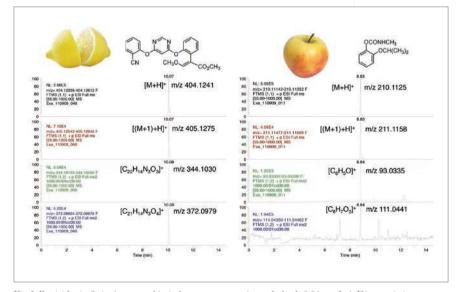
Fig 2. Pesticides in fruits (azoxystrobin in lemon, propoxur in apple, both 0.01 mg/kg). Diagnostic ions (protonated molecule, (M+1) isotope and fragments ions) retrieved from the raw data obtained after HPLC-full scan hrMS analysis. Alternating scan events were performed with and without fragmentation (3).
