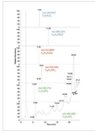
Fig 1. Honey (spiked with various contaminants at 10  $\mu$ g/kg) analysed by HPLC with high resolution MS. Total ion current (TIC) (in black). The individual traces are extracted ion chromatograms (exact mass of [M+H]+ ±5 ppm) of various types of contaminants, from top to bottom: carbendazim, tebuconazole (pesticides), sulfadimethoxine, tylosine (veterinary drugs), atropine, senecionine (plant toxins).
