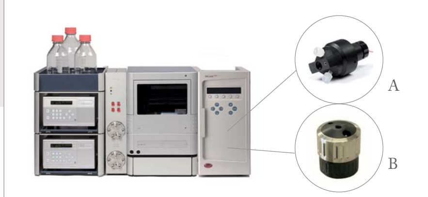
Figure 2. ALEXYS Antibiotics Analyzer for aminoglycosides and macrolides antibiotics analysis, based on RP-HPLC or HPAEC with PAD (3 or 4 steps) detection. Inserts: (A) FlexCell (routine use) and (B) SenCell (in case of EP/USP requirement). Sensitivity FlexCell 100 nmol/L, SenCell 10 nmol/L.
