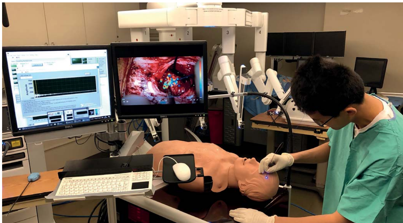
Figure 1. Graduate student Tianchen Sun (Marcu Laboratory, UC Davis) testing the FLIm instrument on the training suit of the UC Davis Medical Center
